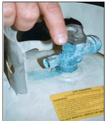
Blue valve means danger!
