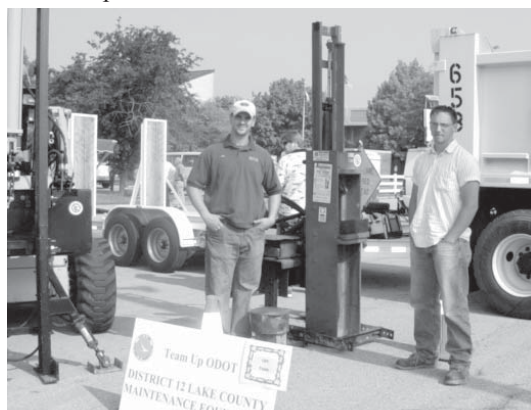
D-12 Lake County workers Joe Hejduk (on left) and brother Sam, standing by the adapted guardrail pounder and custom made post-puller created by Joe which were on display at the 2004 Team Up ODOT event.
